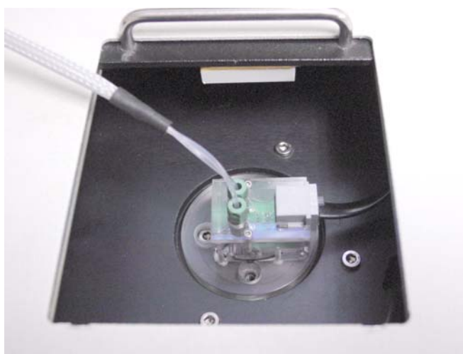
Figure IV- 12: Flow cell inserted into zeta instrument.
