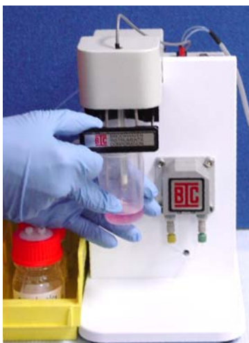
Figure VI- 2: Inserting and removing the sample cup.
